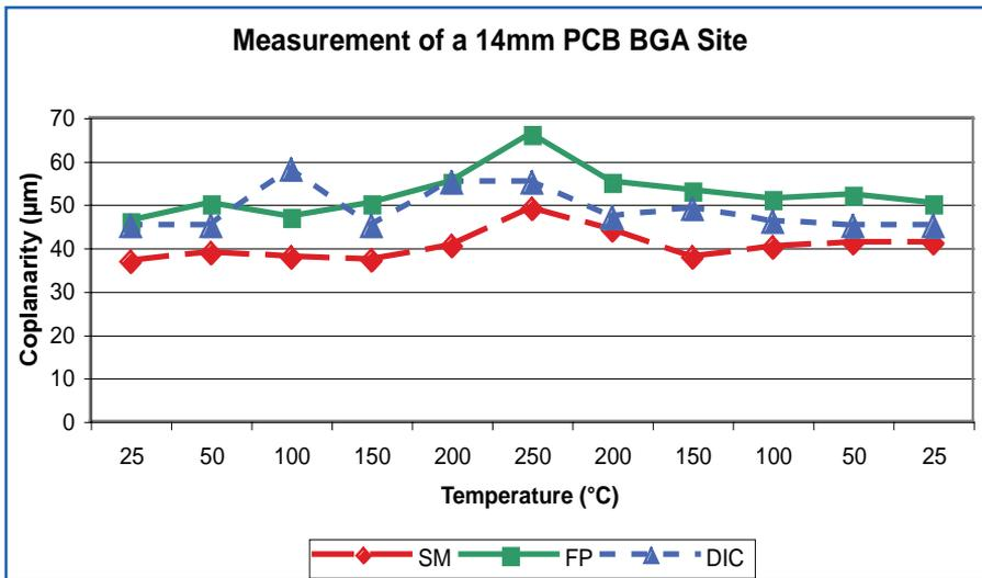
Figure 6b. Thermal warpage of a 14\_14 mm PCB BGA
