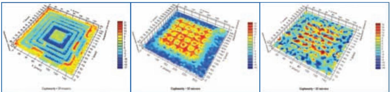
Figure 7. 3D surface plots of a 14mm PCB BGA site at room temperature (a) shadow moiré, full view (b) fringe projection, zoomed view (c) digital image correlation, zoomed view
