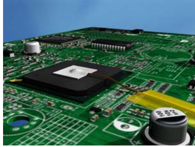
Figure 1a. TC attachment on top of the BGA
