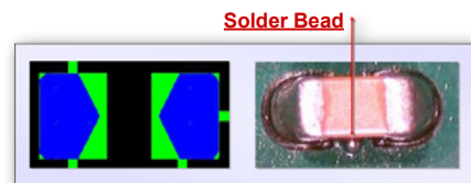
Customized apertures designed to prevent problems such as solder beading
