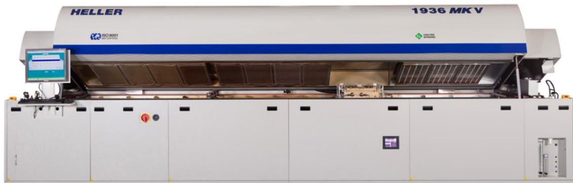
Exhibit 2: Conventional reflow with vacuum chamber module
