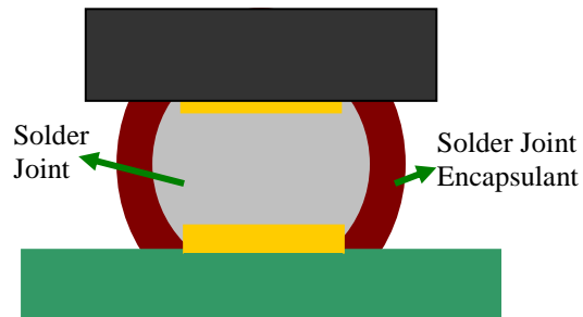
Fig. 2 Schematic cured SMT 266 encapsulated solder joint
