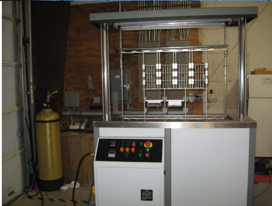
Photo 4 Test Set-up in Lab (squeegees loaded in tool holder)
