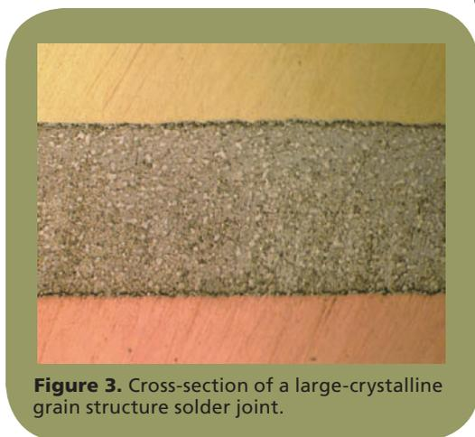
**Figure 3.** Cross-section of a large-crystalline grain structure solder joint.
