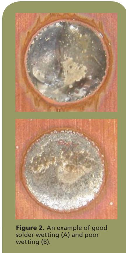
**Figure 2.** An example of good solder wetting (A) and poor wetting (B).
