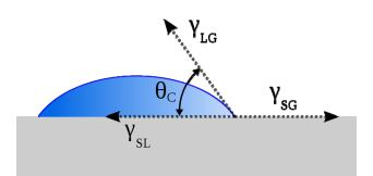
**Figure 1:** The three forces that give rise to contact angles, adapted from [4]
