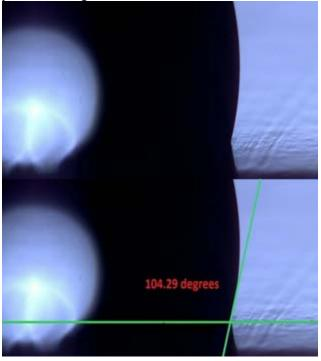
**Figure 4:** Top Half of the Image is the Contact Angle on the Reference Sample – The Bottom Half of the Image is the Contact Angle after Exposure to the Cleaning Agent
