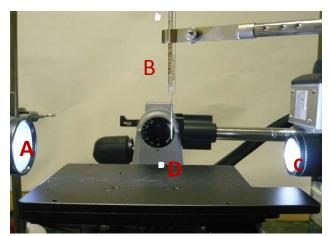
**Figure 3:** Goniometer, A- Light Source, B - 5µL GC syringe, C-Keyence VHX-1000 Camera, D-Sample
