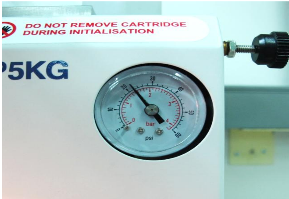
Clamping Pressure: 21 psi
