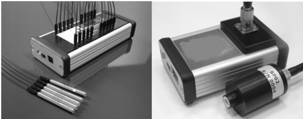
Figure 2: LED Analyser module (a) used for constant monitoring of colour LED colour. The optical probes can be seen in the bottom of the picture, and the Spectrometer module (b) used for reference measurements. We can also see the mini-integrating sphere.
