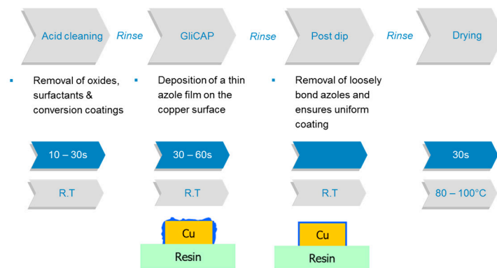
Figure 8. Process steps for the deposition of a thin azole silane film on copper.
