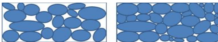
Figure 5 Conductive particles of different shapes and sizes distributed in a printed trace. Left image shows high porosity, less surface contact between particles resulting in a higher resistance trace. Right image shows a higher packing density trace closer to traditional solid PCB trace with lower resistance
