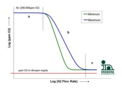
reduce the level but will produce large variations (b). Finally, given a high-enough flow rate, the oxygen concentration will reach a plateau (c) where the minimum oxygen level possible is reached, but turbulent mixing is still introducing some oxygen from the outside air. As you increase the nitrogen flow rate, you are simply increasing the turbulence, and hence the rate of mixing.
