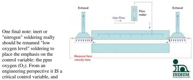
ppm levels within reflow ovens should be measured on a continuous basis.
