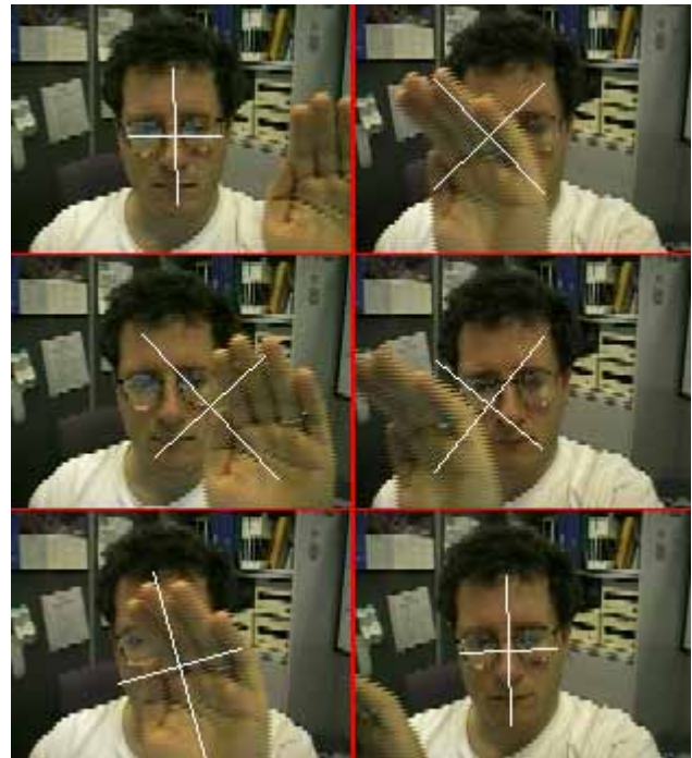
Figure 18: Tracking a face in the presence of passing hand occlusions (sequence: down left then right columns)
