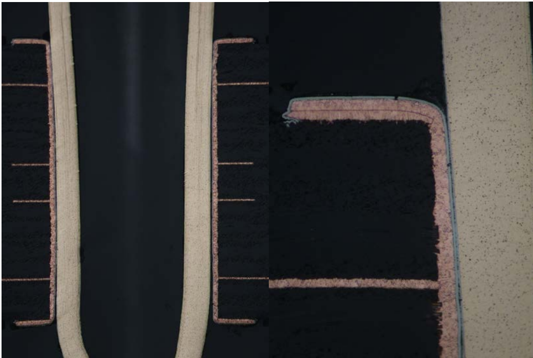
Figure 61 – Vertical cross sectioning of reference connector D, ENIG plating.
