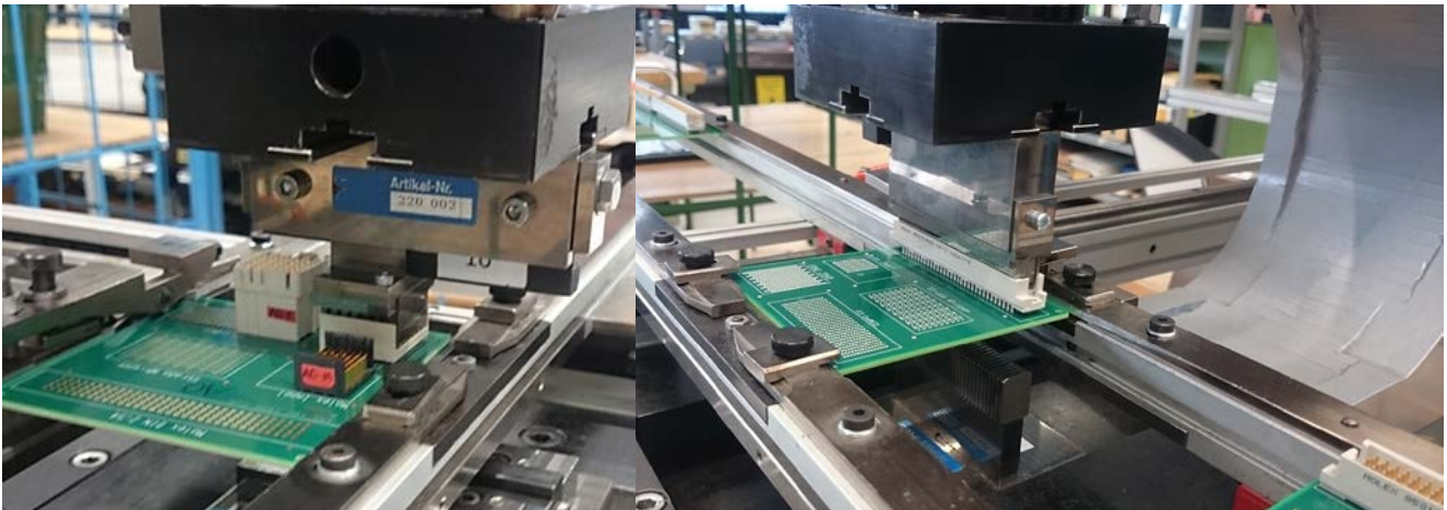
Figure 24 –Press in of the connector A(left) and D (right) during the rework test.
