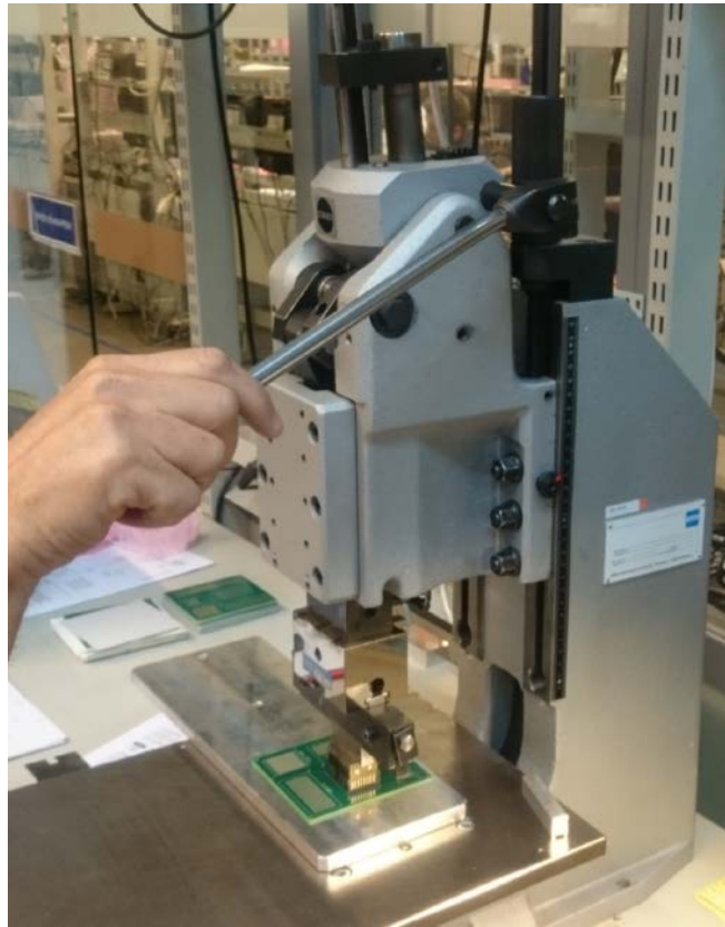
Figure 26 –Manual press in of connector E.
