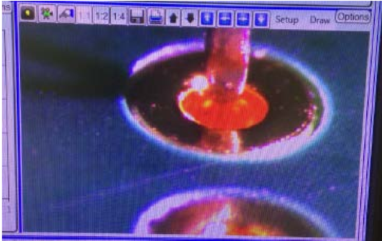
Figure 41 –Vision system used to align pin to center of hole.
