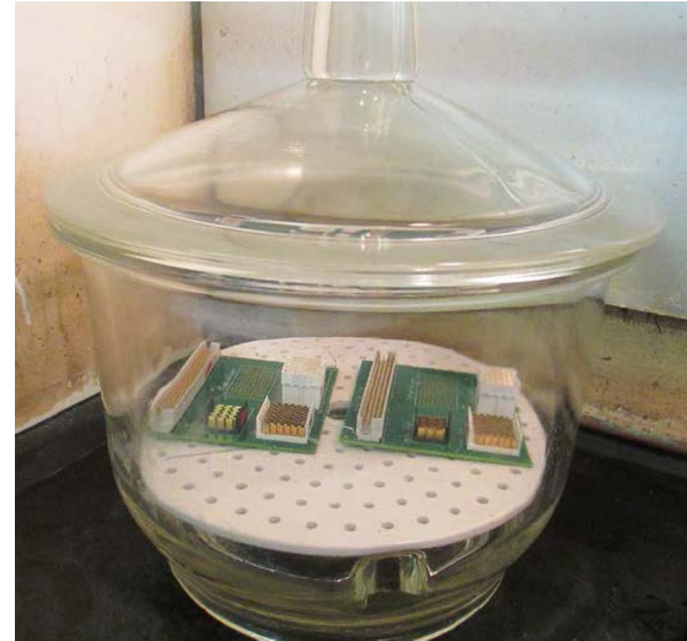
Samples inside test chamber saturated with nitric acid.
