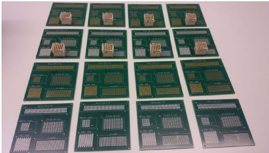
Figure 37 –Boards where connector B had been reworked 0 to 3 times ready to be sent to gas tightness test followed by cross sectioning (boards with connector B) and to insertion and retention test (boards with no connector).
