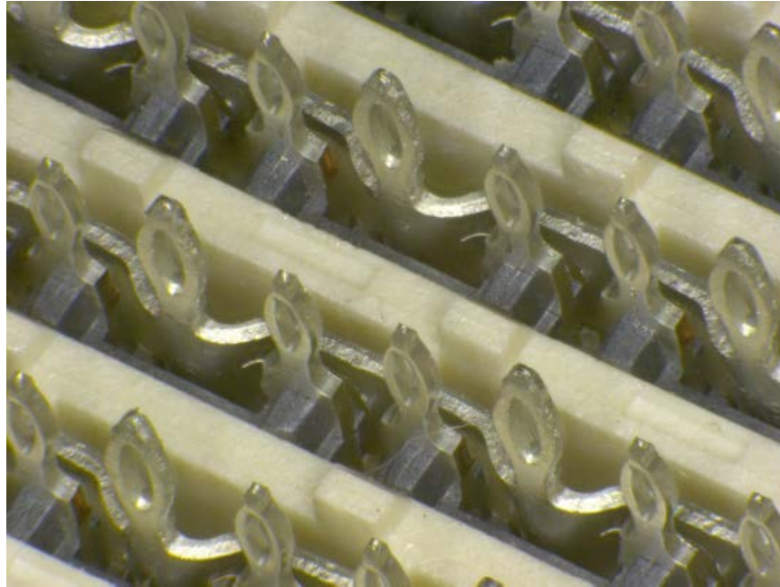
Figure 5 – Press fit pins for high speed connector B.
