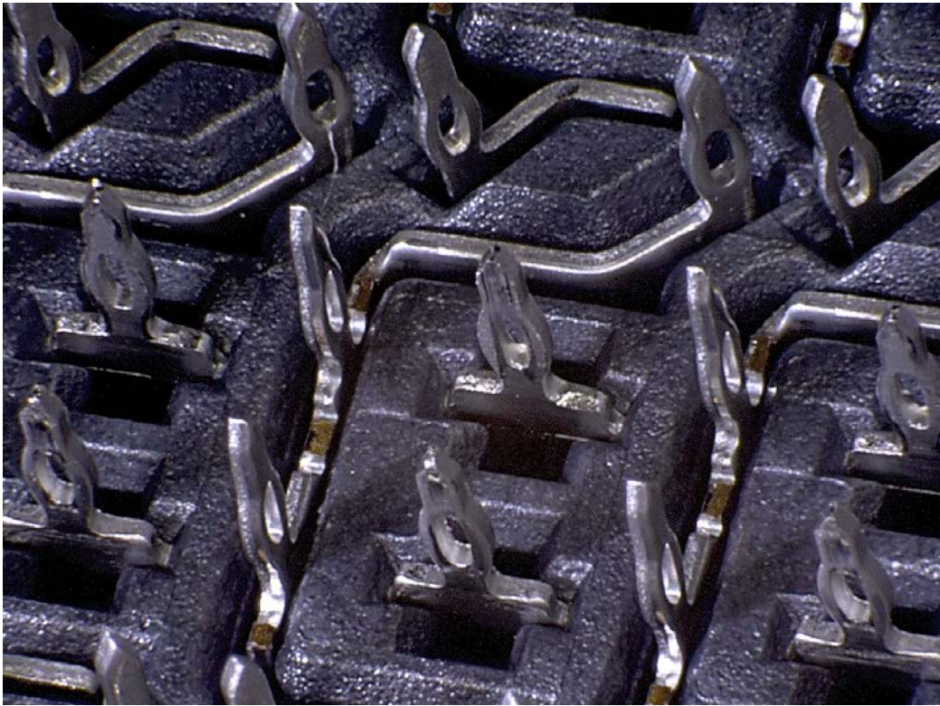
Figure 12 – Press fit pins for high speed connector E.
