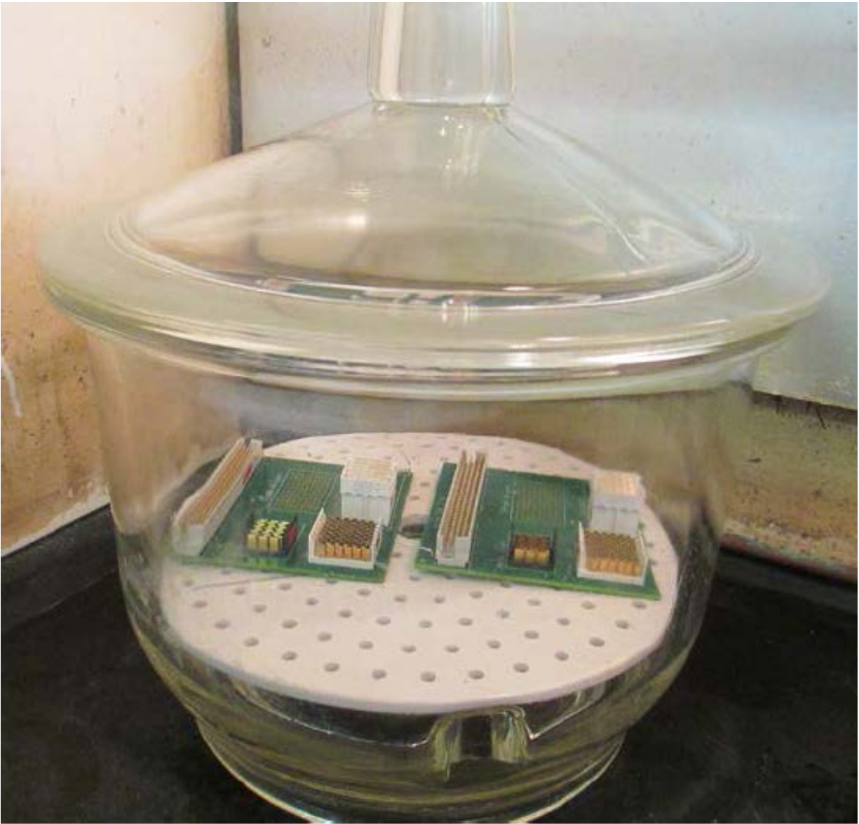
Figure 51 – Samples inside test chamber after nitric acid saturation.
