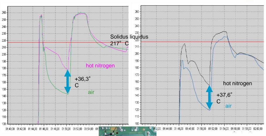
Temperature measurement on small diode pin
