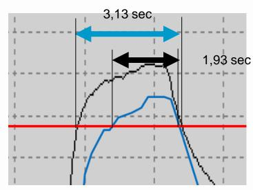
Temperature measurement on small diode pin (+ 25% equivalent contact time)
