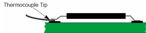
Fig.3. It is best to attach the thermocouple tip between a PCB pad and the corresponding component lead.
