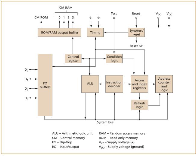
Figure 2. Block diagram of the 4004.
