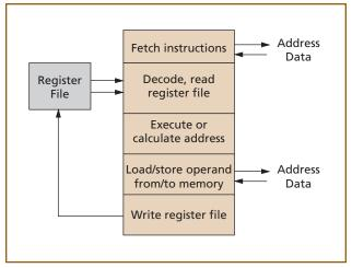
Figure 6. Basic five-stage processor pipeline.
