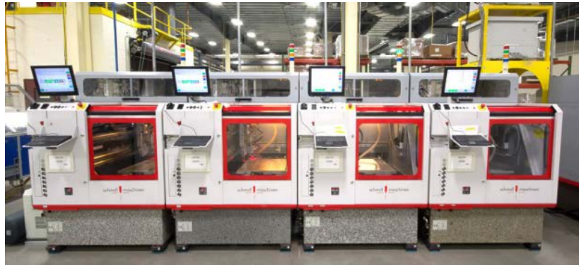
FIGURE 14 – Multi-purpose drill/rout single-station systems with cameras and loaders/unloaders.
