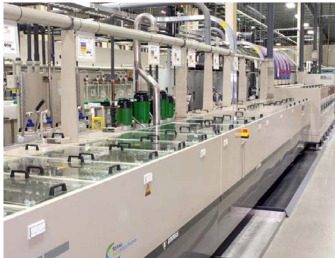
FIGURE 11 - Horizontal conductive polymer metallization.
