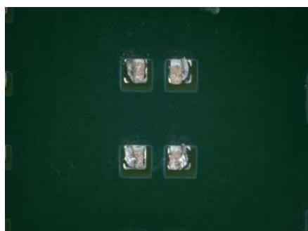
Figure 34 - Underneath 0603 Component After Cleaning using pH neutral
