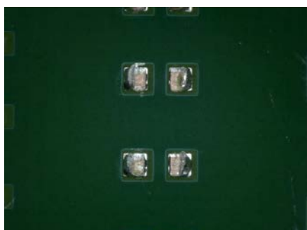
Figure 33 - Underneath 0603 Component After Cleaning using DI-water
