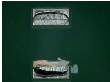
Figure 30 - Underneath 1812 Component After Cleaning using pH neutral
