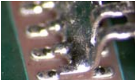
Figure 6 B: Close up of multi-lead bridging on a QFP
