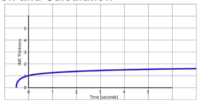
The role of intermetallic compounds (IMC) is critical to the successful formation of a solder joint. With too little IMC formation, typically <0.25  $\mu$ m, the solder joint is cold or dry, which hinders electrical connection. Too much IMC, typically >4 $\mu$ m, solder joint embrittlement becomes a factor.
