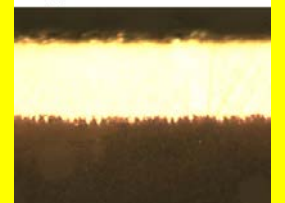
Copper-Dielectric Interface 50x
