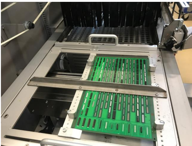
Figure 13: The test-board positioned in the pallet with a bar to keep it flat.
