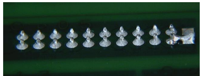
Figure 8: Fine pitch leads with solder thief at the end,
