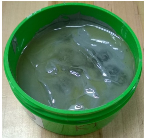
Figure 3: Flux Separation - Halogen-Containing Paste Stored @ RT for 91 Days
