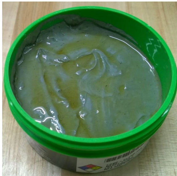
Figure 2: Flux Separation - Halogen-Free Paste Stored @ RT for 91 Days
