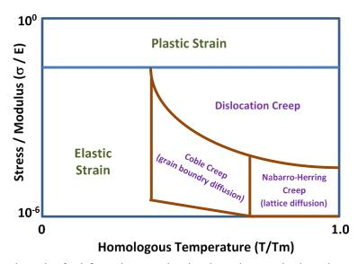
Figure 2: A representative schematic of a deformation map showing the various mechanisms that can induce damage during cyclic fatigue
