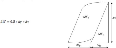
Figure 4: Representative schematic of a solder joint hysteresis loop<sup>19</sup>
