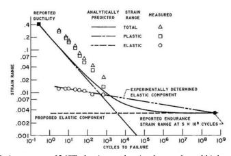
Figure 1: Fatigue curve of 24ST aluminum, showing low cycle and high cycle fatigue<sup>6</sup>
