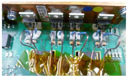
Figure 9: Thermocouple placement on Gate Drive Resistors
