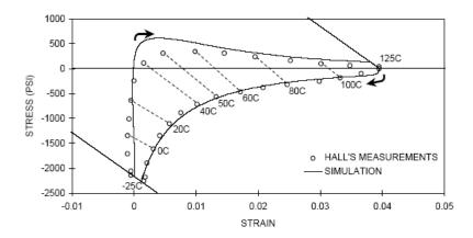
Figure 3: Hysteresis loop of a leadless ceramic chip carrier solder joint during thermal cycling between -25°C and 125°C<sup>16</sup> (obtained through http://www.msed.nist.gov/solder/clech/Sn-Pb\_Creep.htm)
