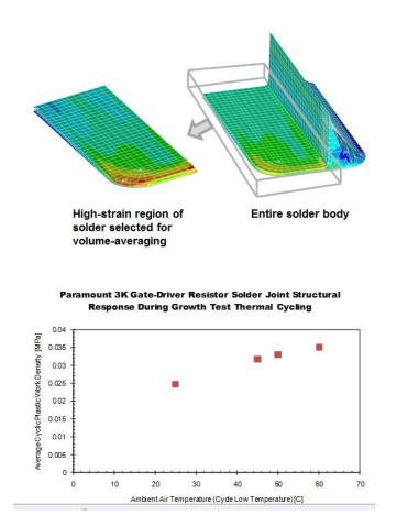
Figure 12: FEA model and estimate of  $\Delta$ Wave
