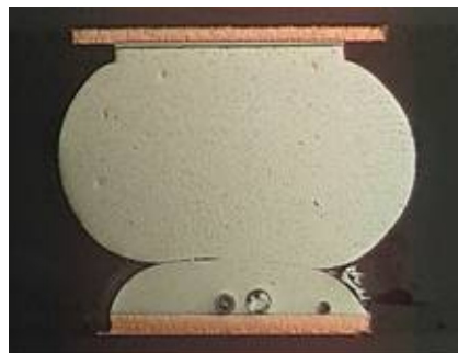
Figure 1: Head in Pillow component soldering defect
