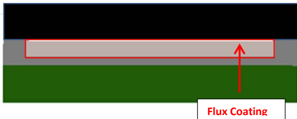
Figure 6. To minimize voiding the solder preform must be flux-coated as shown
