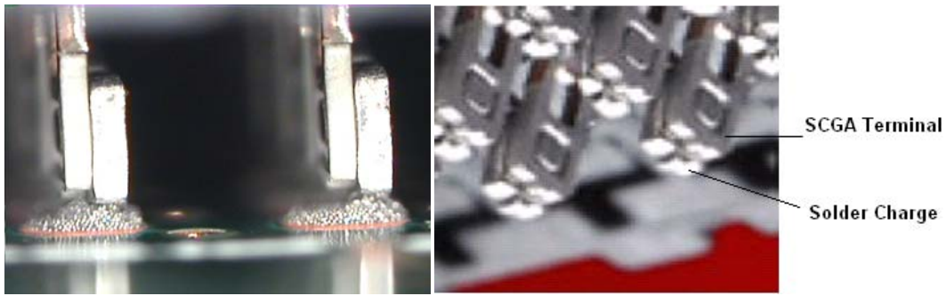
Figure 2: Solder Charge location on Terminal
