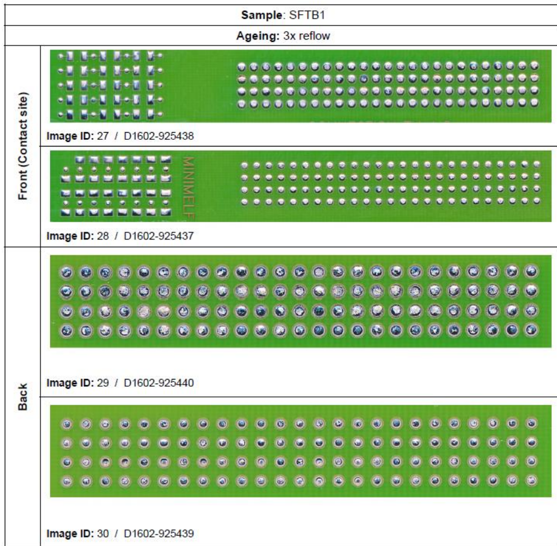
Figure 9: Result for selective wave soldering after 3 x reflow
