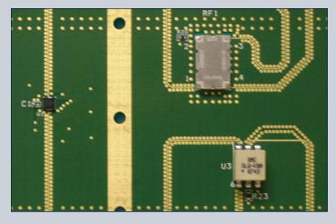
Figure 1: Section of test vehicle with digital attenuator and couplers.
