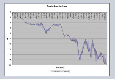
Figure 2: SMT Coupler X Band insertion loss before and after vibration testing.
