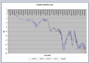
Figure 3: SMT Coupler X Band insertion loss before and after thermal cycling.
