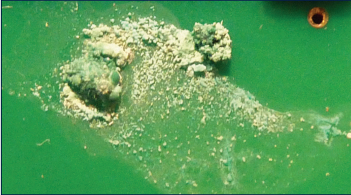
Figure 2: Optical micrograph of green residue residing on board assembly.
