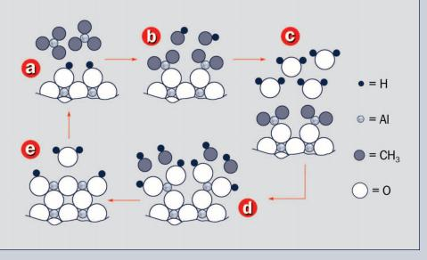
Figure 1: Five-step cycle (a through e) to produce one monolayer of alumina ceramic  $(AI_2O_3)$ . Courtesy of Sundew Technologies, LLC.
