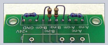
Figure 2: Image of ALD coated through hole components soldered to a board with the solder wetting up to the coated area. Image courtesy of Sundew Technologies, LLC.
