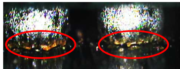
Figure 7: Pad lifting – PBGA676 (SAC405) – 200TS
