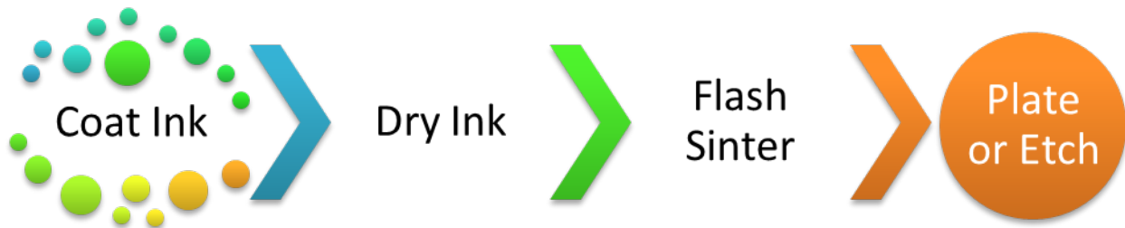
Figure 1. A process for preparing very thin copper foil on polyimide.
