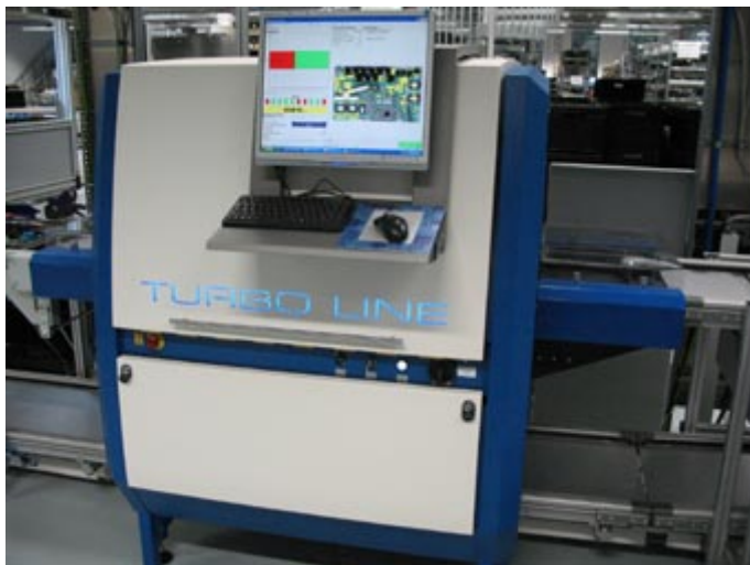
Image 4: OptiCon TurboLine with low-flow return conveyor
