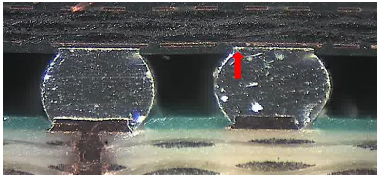
Figure 7 Solder joint image prior to separation, the dog-bone joint at the right side showed an upward pushing
