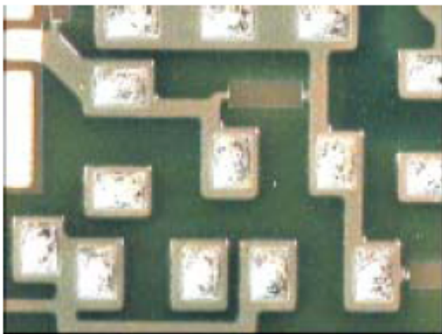
Figure 6 F540Ag35 Reflow in Nitrogen
