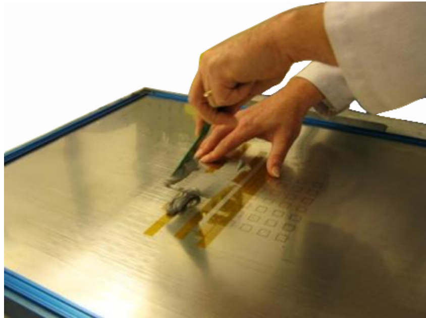
Figure 19 – Manual screenprinting of solder paste on bottom side of stencil.
