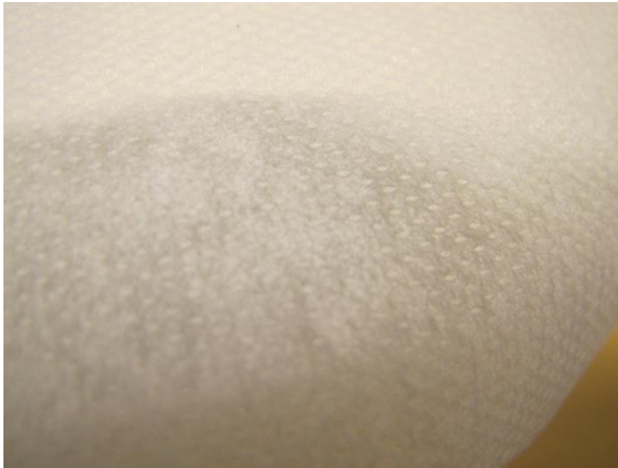
Figure 7 – Photo of cleaning paper B. Wave formed surface because of regular imprints.
