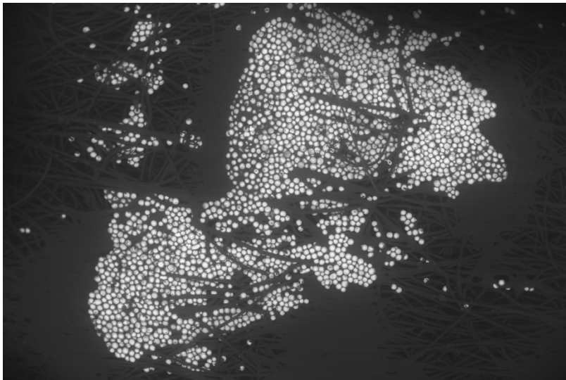
Figure 24 – Cleaning paper B, entrapped solder particles.
