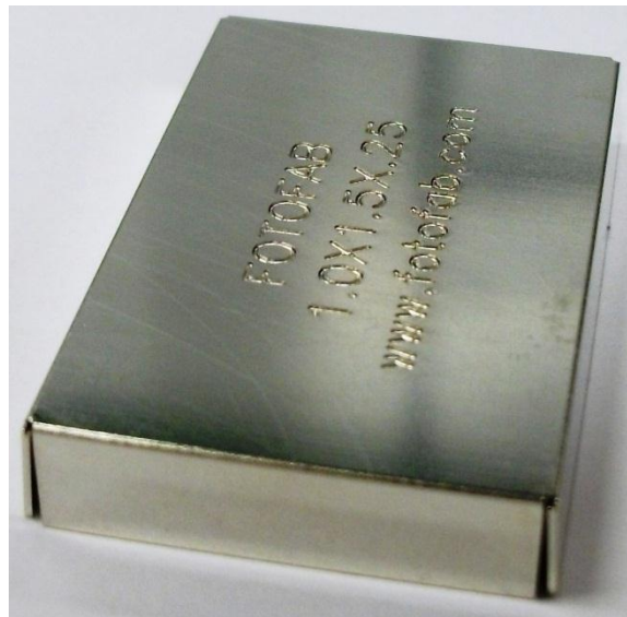
Figure 2 - Folded RF Shield
