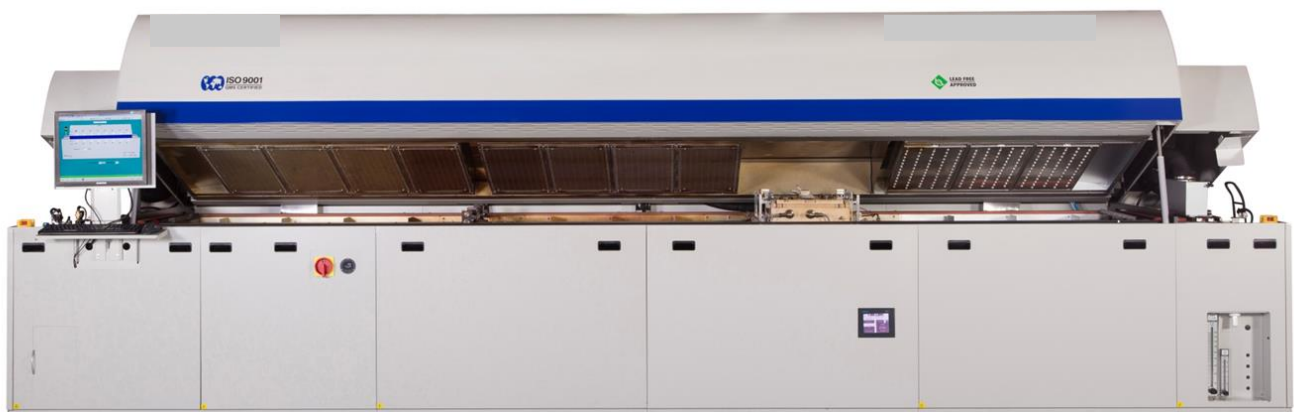
Figure 6- Eight Heat Zone Convection Oven with Vacuum Chamber in between Heat and Cooling Zones
