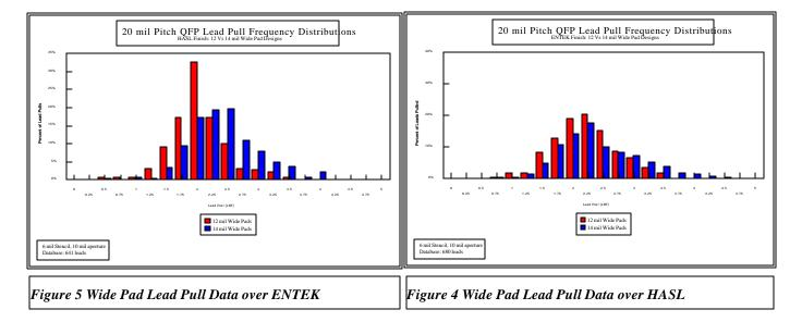
Although side fillets on fine pitch leads may contribute very little to joint integrity they do ensure that the full benefit of the heal fillet is realized. The frequency distributions below illustrate the subtle increase in joint strength by the shift of the frequency distributions for both ENTEK and HASL board finishes. Technical Bulletin *finepads.pdf* provides fine pitch (0.8 to 0.5mm) guidelines based on actual designs and process studies and supported by the IPC design guidelines.
