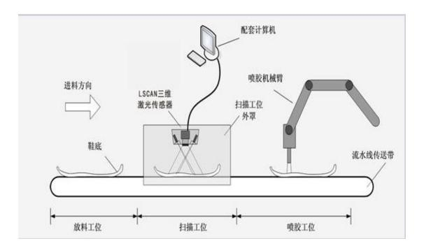
Intelligent operation advantage manual only need general operation can be automated workshop, mechanical arm automatic spraying glue, accurate spraying, reduce glue waste. Environmental protection effect of long-term close contact with glue seriously affects human health and mechanical work, glue does not directly contact, do not harm the human body.
